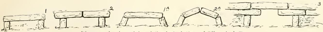
Diagrams showing origins of Simple Arch (2A) and Off-set Arch (3).
