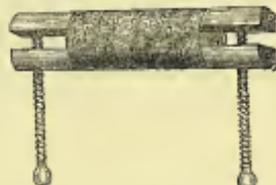
The above engraving will convey a better idea of this little machine than any we are capable of giving. It is used for stretching knitted, netted, and crochet purses.
