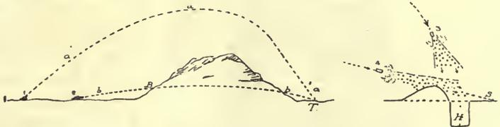
The left-hand picture shows the advantage possessed by a howitzer over a field gun when firing over a hill at some troops at T. 1 is the howitzer, and a, a, a is the track of its shell. 2 is the field gun, and b, b would be the path of its shell were it not stopped at B by the hill.
