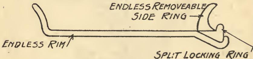
Not removeable from wheel Accepts either straight, side or clincher tires.
