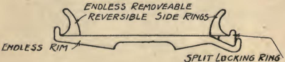
Removeable from wheel. Accepts either straight side or clincher tires.
