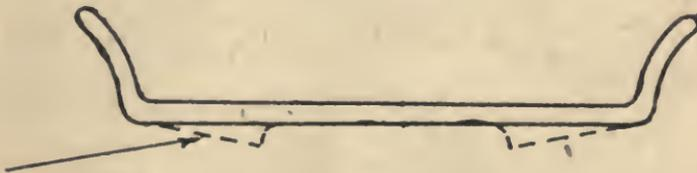
Rim may or may not have taper indicated by dotted line. A one-piece ring, usually split transversely. Rim is removeable from wheel, and held in place by several wedge clips, or by wedge ring and forcing clips.
