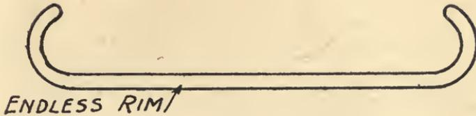
An endless one-piece rim, shrunk direct to wheel, or held direct by spoke nipples on wire wheels.
