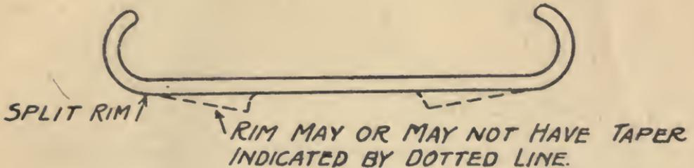
A type removeable from wheel, held in place by several wedge clips, or by wedge ring and forcing clips.
