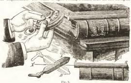
brought before the magnet, and its V o'clock vibrated before the south pole till this south magnetism disappears; in other words, produces no deflection on the needle of the magnetometer. An examination of the magnetism of the watch before the magnetometer gives the following results:
