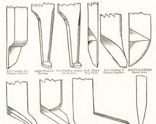
Round-ended for Turn-Ing Heavy Shafting. Diamond-point for Turning Small Shafting. Turning Tools.
