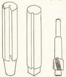
Single Lipped Single Lipped Counter Boring Reamer. Tool.
